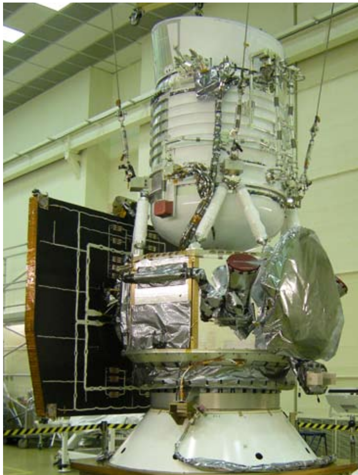
The WISE flight system at Ball Aerospace in Colorado.
