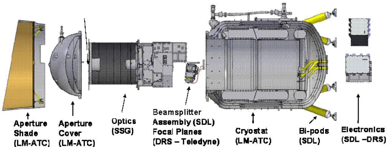
**Figure 4 Payload Subsystems and Key Components**
