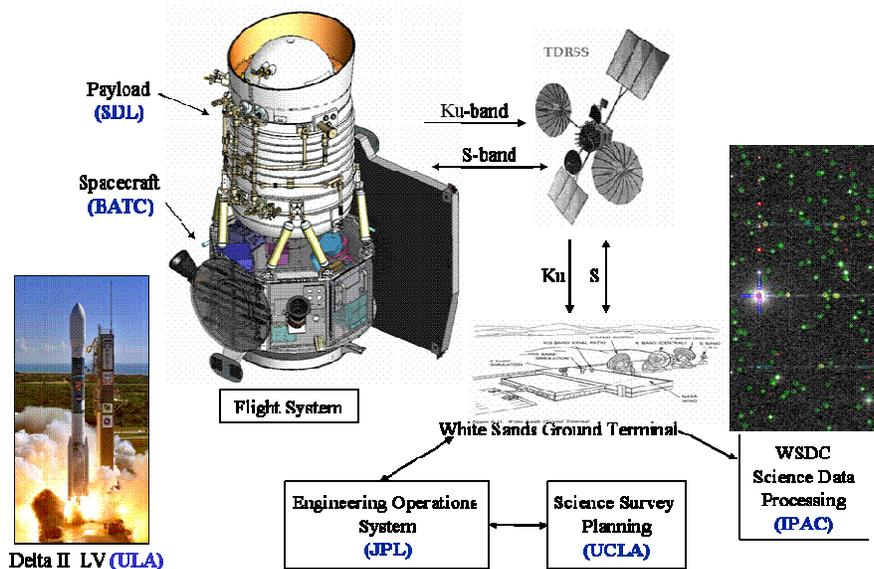
**Figure 1 WISE Mission Elements and Operation Concept**
