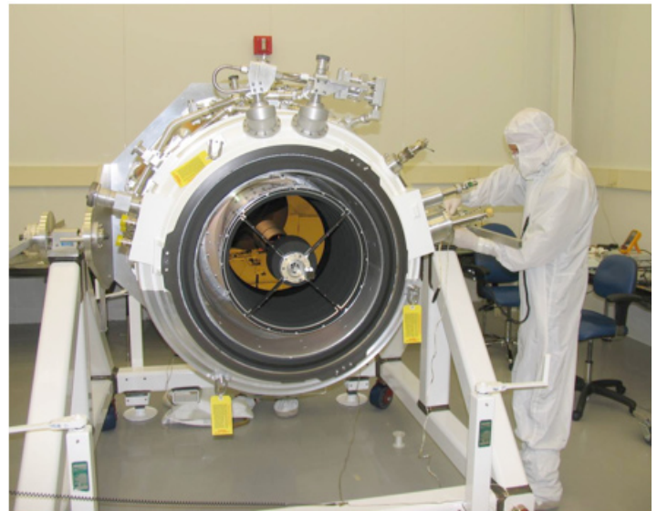
The WISE payload showing the telescope with cover removed, during assembly at the Space Dynamics Lab in Utah.
